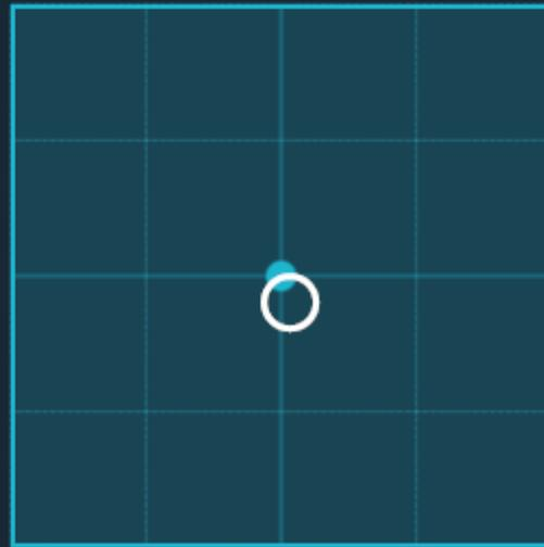
Clip the sensor on the stand or another stable object(e.g. KAT loco box) and put it on the ground with the light up. Stabilize it for the white circle to reach the screen center.
