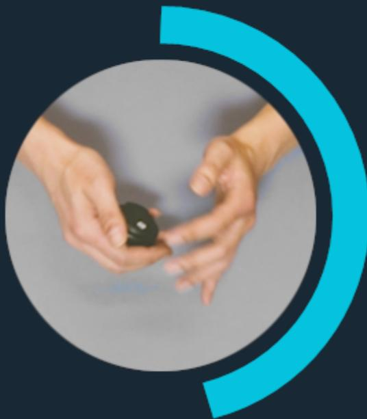
Continuously toss the waist sensor from one hand to another until the magnetic data collection process is finished. Progress is represented by the blue circle.
